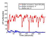
Fig. 21. Buffer size and occupancy time histories measured at the AP with fixed 400-packet buffers and the A\* algorithm.
